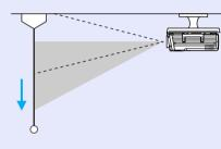
• If correct adjustment cannot be obtained using the lens shift function, extend the front adjustable feet to tilt the projector. p.51 When the projector is tilted, keystone distortion may appear in the projected images. If this happens, you can correct this keystone distortion. p.52
