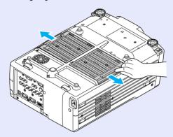
Remove the old air filter that is in the air filter cover.
