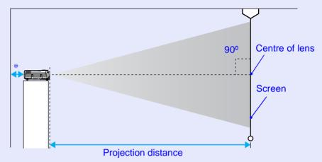
\* When installing against a wall, leave a space of 20 cm (7.9 in.) or more between the projector and the wall.
