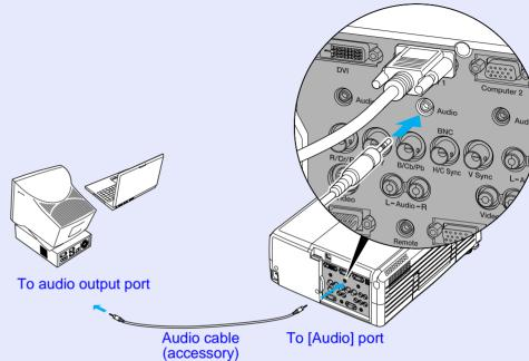
\* An accessory audio cable is not supplied with the EMP-9300. Use a commePrcially-available audio cable instead.
