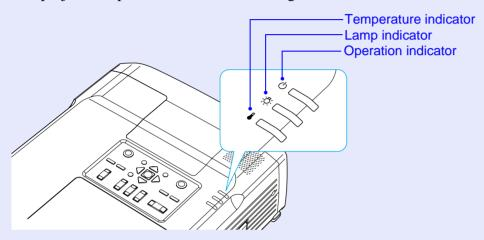
The following tables show what the indicators mean and how to remedy the problems that they indicate. If both indicators are off, check that the power cable is connected correctly and that power is being supplied normally.
