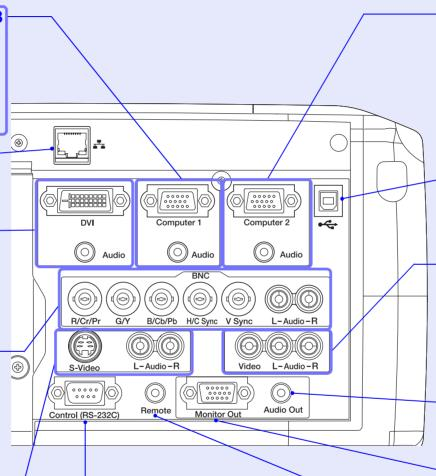
• [Control (RS-232C)] port p.147 Connects the projector to a computer using an
