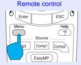
2 Select "Reset Lamp Timer" from the "About" menu and then press the [Enter] button on the remote control or the [Auto/Enter] button on the projector's control panel.
