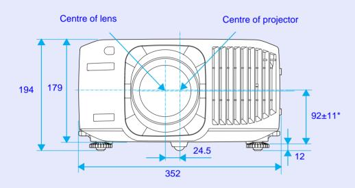
\*Distance from center of lens to suspension bracket fixing point (The centre of the lens moves vertically when using the lens shift.)
