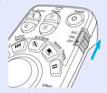
Point the remote control light-emitting area towards one of the remote control light-receiving areas on the projector and operate the remote control buttons.
