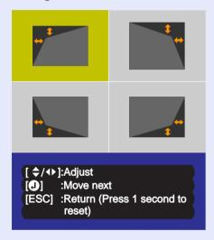
Press the [Enter] button on the remote control or the [Auto/Enter] button on the projector's control panel to select the correction angle in the screen.
