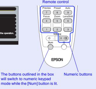
Use the numeric keypad buttons to enter the password that has been set. If the password is entered correctly, projection will then start.
