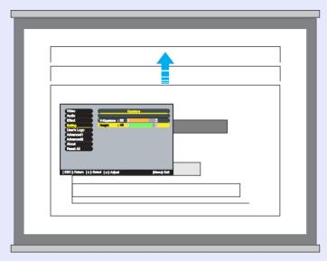
When the adjustment is complete, press the [Menu] button on either the remote control or the projector's control panel to close the configuration menu.
