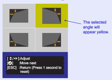
Tilt the [○] button on the remote control, or press the [Sync +], [Sync -], [Tracking +] and [Tracking -] button on the projector's control panel to correct the angle position.
