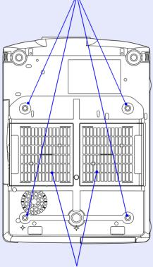
• Air filters (2 places) (air intake vents) \_ p.130, p.136 Prevent dust and other foreign particles from being drawn into the
