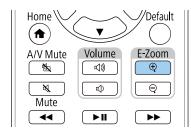
The projected image is enlarged focusing around the center of the image. You can enlarge the image between one to four times in 25 incremental steps.
