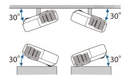
If you use the projector tilted at an angle of more than 30  $^\circ$  it could be damaged and cause an accident.
