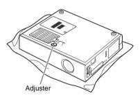
2 Slide switch A in the slit in front of the adjuster in the direction of the arrow (toward the front panel of the projector) with the small minus screwdriver.
