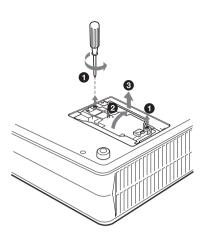
**4** Insert the new lamp all the way in until it is securely in place. Tighten the screws. Fold the handle.
