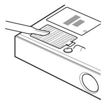
When it becomes difficult to remove the dust from the filter with a vacuum cleaner, remove the air filter and wash it.
