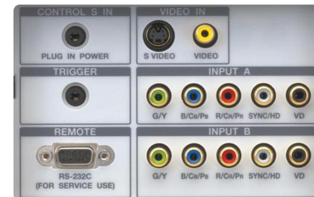
**Versatile Inputs:** rear connector panel gives you inputs for standard (composite) TV and video equipment, S-Video high-resolution components, RGB/Component video sources, RS-232C control systems, and Control S for home entertainment component integration.
