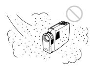
Avoid installing the unit in a location where there is a lot of dust; otherwise, the air filter will be obstructed. The dust blocking the air through the filter may cause raising the internal heat of the projector. Clean it up periodically.
