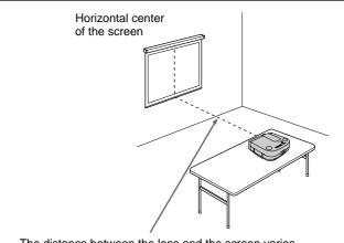
The distance between the lens and the screen varies depending on the size of the screen. Use the following table as a guide.
