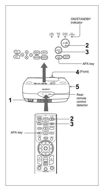
1 After all equipment is connected completely, plug the AC power cord into the wall outlet.
