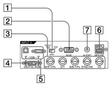
1 DIGITAL RGB/5BNC/RGB switch: Selects DIGITAL RGB, 5BNC or RGB on INPUT A connectors. Select the appropriate position depending on the input signal.
