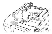
5 Insert the new lamp all the way in until it is securely in place. Tighten the screws. Fold down the handle.
