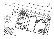
4 While holding the handle and keeping the lamp unit horizontal, pull straight up.
