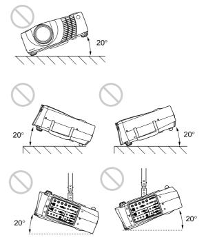
Avoid using as the unit tilts more than 20 degrees. Do not install the unit other than on the floor or ceiling. These installation may cause malfunction.
