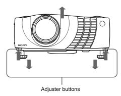
While pressing the buttons, lower the projector. Then, release the buttons.
