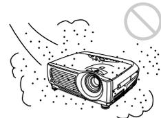
Avoid installing the unit in a location where there is a lot of dust; otherwise, the air filter will clog. The dust blocking the air through the filter may cause the internal heat level of the projector to rise. Clean the filter periodically.
