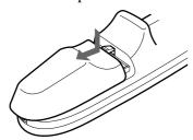
**2** Install the two size AA (R6) batteries (supplied) with the correct polarity.
