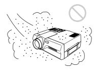
Avoid installing the unit in a location where there is a lot of dust; otherwise, the air filter will be obstructed. The dust blocking the air through the filter may cause raising the internal heat of the projector. Clean it up periodically.
