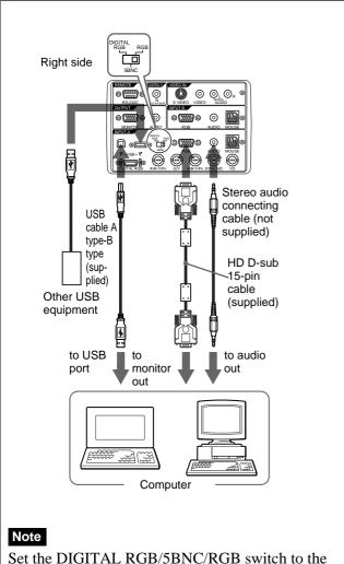
Set the DIGITAL RGB/5BNC/RGB switch to the suitable position depending on the connection.
