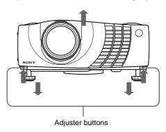
**2** While pressing the buttons, lower the projector. Then, release the buttons. For fine adjustment, turn the adjusters to the right and the left.
