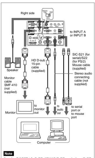
Set the DIGITAL RGB/5BNC/RGB switch to RGB (right) when you connect the computer to the INPUT A connector.
