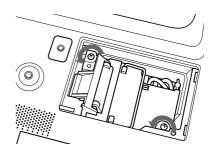
4 While holding the handle and keeping the lamp unit horizontal, pull straight up.
