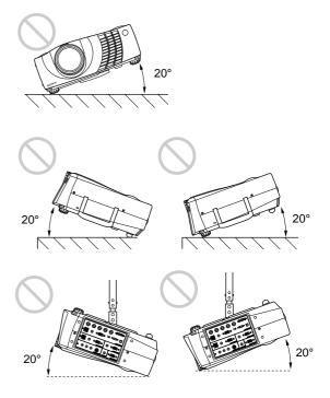
Avoid using as the unit tilts more than 20 degrees. Do not install the unit other than on the floor or ceiling. These installation may cause malfunction.
