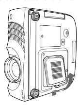
**3** Peel off the air filter. (The air filter is secured with Velcro tape (3).)
