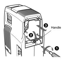
5 Insert the new lamp all the way in until it is securely in place. Tighten the screw. Fold up the handle.
