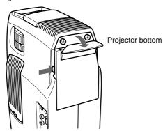
**3** Open the lamp cover that is a part of the adjuster by loosening two screws with the Philips screwdriver (supplied with the LMP-P120 Projector Lamp).
