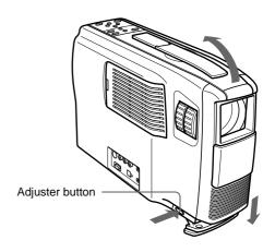
**2** While pressing the button, lower the projector. Then, release the button.
