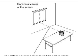
The distance between the lens and the screen varies depending on the size of the screen. Use the following table as a guide.
