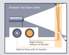
The automatically adjusting iris diaphragm – an important component of the SANYO TOPAZreal technology – ensures that the contrast and depth of projected images is increased at those crucial moments.
