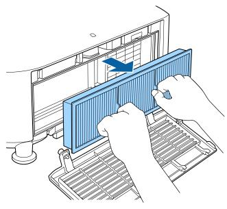
Tap each side of the air filter 4 to 5 times to shake off any excess dust.
