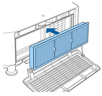
**8** Replace the air filter cover as shown and tighten the screws.
