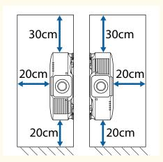
• Do not install the projector in a location that does not allow air to circulate, such as on a shelf or in a box.
