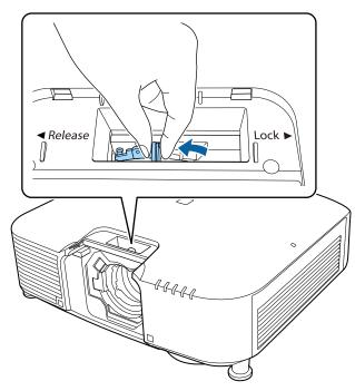
Insert the lens straight into the projector's lens socket with the white dot facing up.
