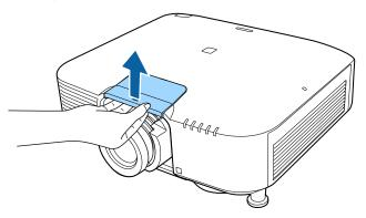
4. Remove the stopper, if necessary.
