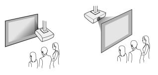
Select the correct **Projection** option in the projector's **Installation** menu according to the installation method being used. If necessary, turn on the **Inv Direction Button** setting in the projector's **Operation** menu and adjust the **Menu Rotation** setting in the projector's **Display** menu.
