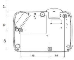
Ceiling mount screw: M4 x 8 (Max L = 25 mm; L = 20 mm)
