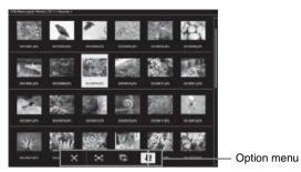
Press the 4/4/4 key on the remote commander to select an image, then press the ENTER key. The option menu appears in the lower part of the screen.
