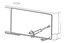
3 Loosen the 3 screws on the lamp (1) then pull out the lamp by its grab (2).
