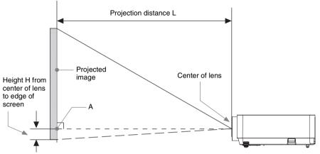
\* The number will be minus when the bottom of the projected image is lower than A.
