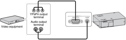
Audio cable (Phono plug  $\times 2$  – stereo mini plug) (not supplied)
