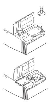
**5** Loosen the 3 screws on the lamp with the Phillips screwdriver. Hold up the handle, then pull the lamp straight out.
