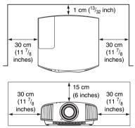
Air from air conditioners or the ventilation holes of this unit or other devices, may cause oscillation on the screen. Be sure not to install this unit in the area where the air from air conditioners or the ventilation holes of these devices reach to the front side of this unit.
