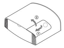
**4** Loosen the lamp door (inner cover) screw with a Phillips screwdriver, and then open the lamp door.
