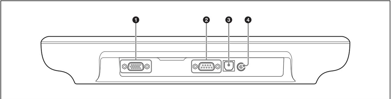
**1 VGA connector (D-sub 15 pin, female)**
