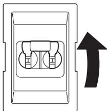
The power will turn on and the MAIN indicator and LIGHT indicator will turn solid red when the projectors enter standby mode.
