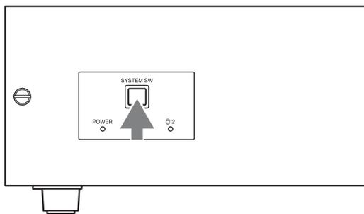
The POWER indicator will blink green, and after start-up is complete, it will turn solid green. Once the server is on, the "Login" screen will be displayed on the monitor.
