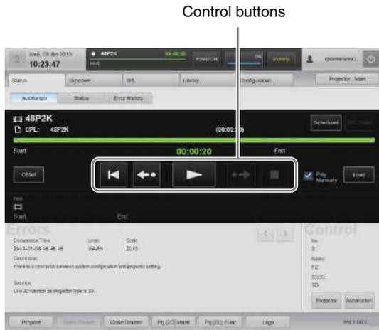
During CPL playback, the playback progress is displayed on the progress bar.
