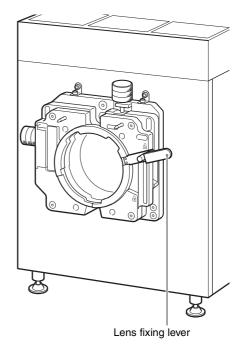
**2** Attach the lens to the projector while firmly holding the lens not to drop it and aligning the position.
