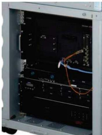
Server and SMS system is enclosed within the projector
