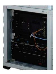
Server and SMS system is enclosed within the projector Above are (top to bottom) LMT 100 media Block SMS computer Two Terabyte Raid system for content storage
