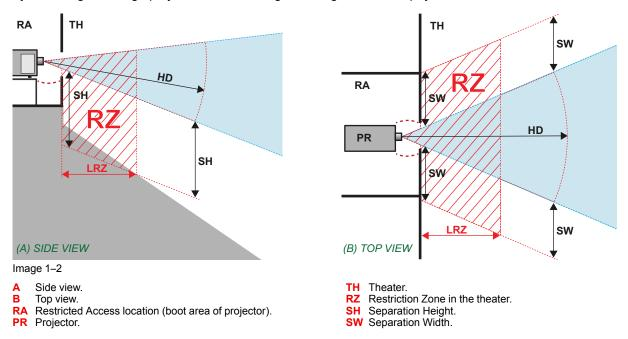
Based on national requirements, no person is allowed to enter the projected beam within the zone between the projection lens and the related hazard distance (HD). This shall be physically impossible by creating sufficient separation height or by placing barriers. The minimum separation height takes into account the surface upon which persons other than operator, performers or employees are permitted to stand.
