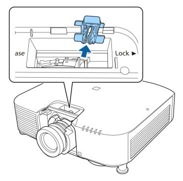
Hold the lens firmly as you pinch the lock lever and move it to the **Release** position.
