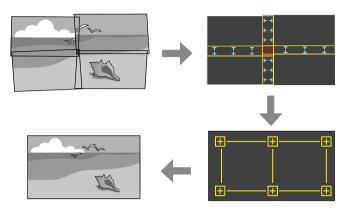
You can easily and quickly create a single seamless image from multiple projectors when projecting on a flat screen.
