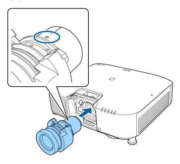
Hold the lens firmly, then pinch the lock lever and move it to the **Lock** position.
