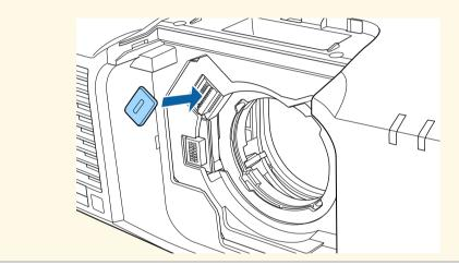
Insert the lens straight into the projector's lens socket with the white dot facing up.
