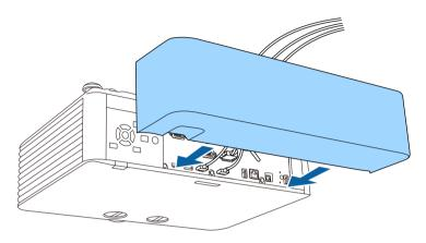
**3** Tighten the cable cover screws.
