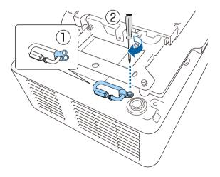
2 Loop the safety wire through the hole in the ceiling mount, and then attach both ends to the carabiner.
