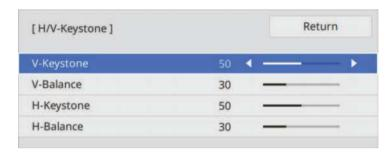
Use the arrow buttons on the projector or the remote control to select between vertical and horizontal keystone correction and to adjust the image shape as necessary.
