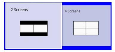
When splitting screen into halves, the currently selected input source moves to the left of the screen.
