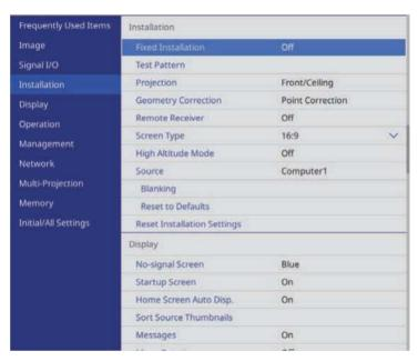
Select **Geometry Correction** and press [Enter]. You see the **Geometry Correction** screen.
