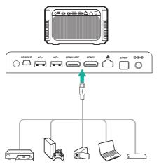
2 Press **SOURCE** to access and select *HDMI* 1 or *HDMI* 2 input source.
