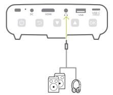
When connecting to the headphones, use the volume control on the remote control (or on the projector) to adjust the volume to a comfortable level
