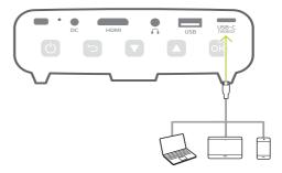
2 If the projection screen does not show images, select USB-C input. Press ♣ on the remote control to access the settings menu, then navigate to select USB-C.
