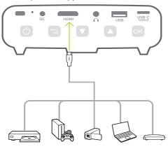
2 If the projection screen does not show images, select HDMI input. Press ☆ on the remote control to access the settings menu, then navigate to select HDMI.
