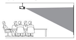
To adjust projection to the correct position, press on remote control to access the settings menu, then navigate to select Projection Mode - Rotate Ceiling, then press OK.
