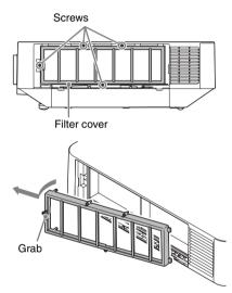
**5** Pull out the air filter from the main unit.
