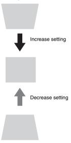
Press the RESET key to restore the projected image before adjustment.\*1
