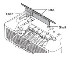
2 Close the terminal cover. Close the terminal cover until the two tabs on the terminal cover click.
