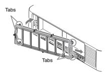
**8** Fit the two tabs on the side cover into place and slide the side cover upward.
