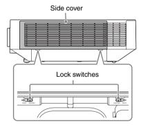
**3** Slide the side cover downward by pushing its upper corners on both sides to remove the side cover.
