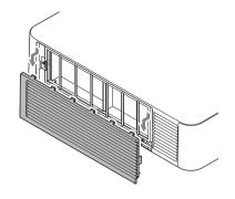
**4** Loosen the screws (four) and pull out the filter cover by pinching the grab on the left side.
