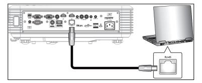
On the PC (Laptop), select Start > Control Panel > Network Connections.
