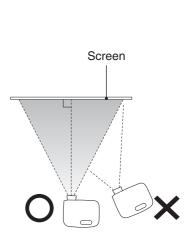
If the projector is placed at an angle to the screen, then the projected image will be distorted.
