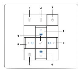
1 LAMP warning light If the LAMP light is solid amber, replace the lamp. If the LAMP light is blinking amber, the projector automatically shuts down indicating a system failure. If this problem persists, contact Dell.
