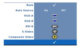
default) to autodetect the available input signals. If you press the Source button when the projector is on, it automatically finds the next available input signal. Select Off to lock the current input signal. If you press the Source button when the Auto Source mode is set to Off, you can
