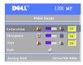
**SATURATION**—Press the (-) button on the control panel or the ◀ button on the remote control to decrease the amount of color in the image and press the (+) button on the control panel or the ▶ button on the remote control to increase the amount of color in the image.
