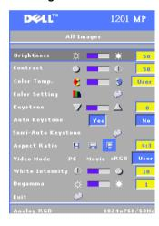
**BRIGHTNESS**—Use the (-) or (+) button on the control panel or the ◀ or ▶ button on the remote control to adjust the brightness of the image.
