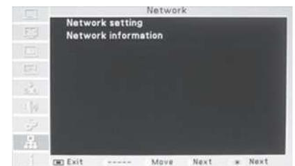
Set DHCP to On: Assign an IP address to the projector from an external DHCP server automatically.
