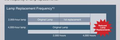
(\*1): When used in Lamp Low mode. Maximum lamp life at standard mode use is 2,000 hours. (\*2): Lamp life refers to the average time required for brightness to be reduced by half, and not the time specified in the warranty. Use time may vary widely the environment and conditions, and whether or not cleaning and other maintenance procedures are followed.
