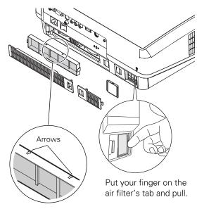
When putting back this air filter, make sure that the arrows on the filter are facing towards the projector.
