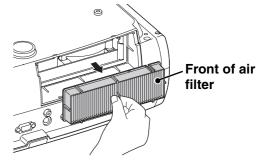
3 Tap the air filter four or five times with the surface facing downwards to shake off the dust.
