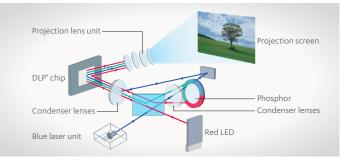
CASIO's unique optical engine combines a laser with an LED. It achieves high luminance by using light from a blue laser converted by the phosphor and the color wheel to complement the red light conventionally projected by red LEDs. The resulting light source realizes high brightness of 4000 lumens.
