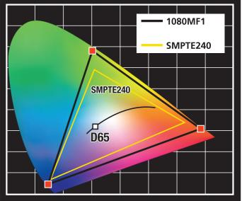
As this diagram shows, the colour gamut of the MF1 comfortably exceeds that of 1080i HDTV (SMPTE240)
