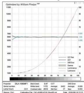
The optimisation process provides accurate colour temperature and Gamma tracking (see above), while the white field uniformity (above right) is superbly aligned for virtually zero deviation for an extraordinarily wide range of luminance values.
