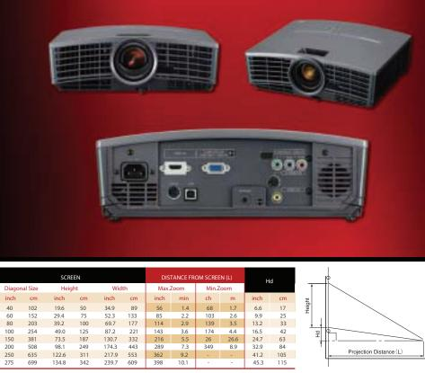
Unit measured in inches. \*Hd is distance from lens axis to image bottom. The above numbers are approximate values.
