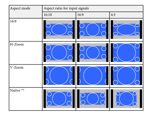
\* When inputting an HDTV signal (720p/1080i/1080p), the aspect ratio of the signal is maintained, while the image is trimmed on the left and right and displayed.
