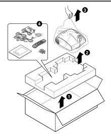
To remove the HT3000 system from its carton follow the diagrams (Fig. 4).
