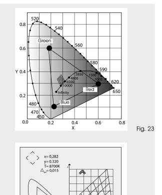
The colour temperature is constant on the vertical lines, but is more or less different from the black body curve. This means that the higher points of the graph are more green. On the contrary, the lower points of the graphic yield a more purple image.
