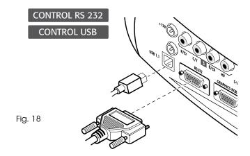
The projector can be controlled from a PC: simply hookup the interface connector to a PC's RS232 serial cable or to a PC's USB 1.1 cable.
