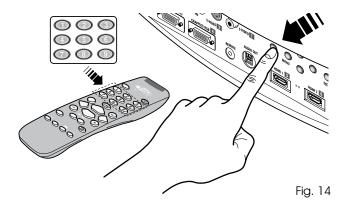
When the unit is switched on from standby the lamp switches on; after a brief period of warming up, the image displays (blue led on). The projected image comes from the input selected when the unit was last switched off (Fig. 14).
