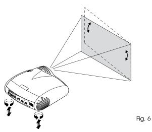
Place the projector at the desired distance from the screen: the size of the projected image is a function of the distance between the lens and the screen and the lens zoom setting. Use the motor zoom (Fig. 7) to zoom the projected image in and out.
