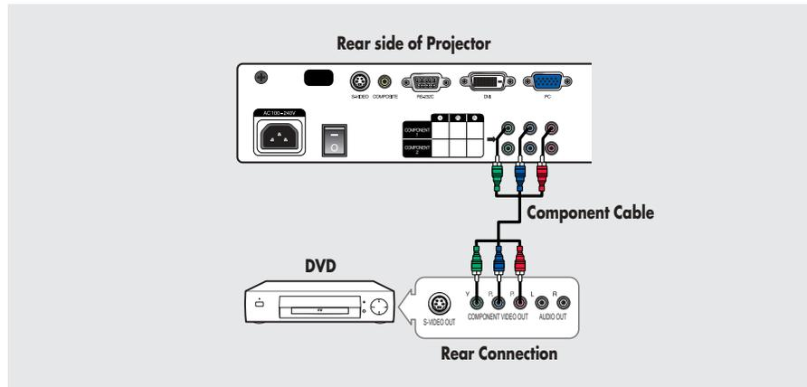
Connect COMPONENT1 or COMPONENT2 (Y/Pb/Pr) ports of the projector to Component port on the rear side of DVD using Component Cable.
