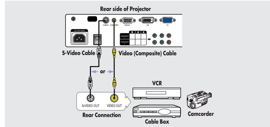
Connect COMPOSITE (yellow) input port of the projector to the VIDEO (yellow) OUT port of video equipment using the video cable.
