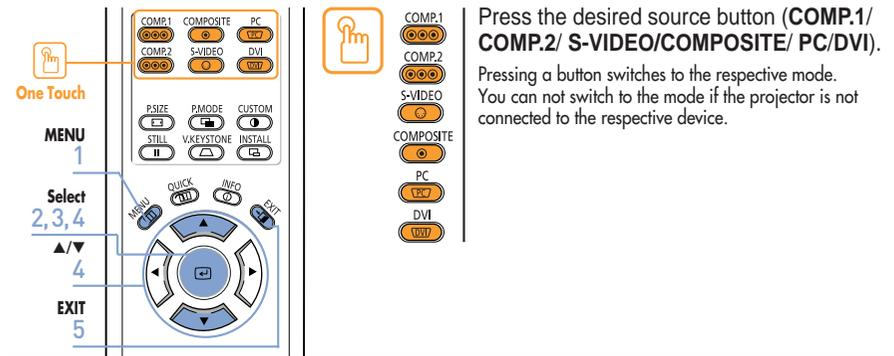
Press the desired source button (**COMP.1/COMP.2/ S-VIDEO/COMPOSITE/ PC/DVI**).
