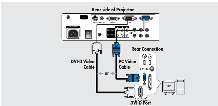
Connect PC (RGB In) port on the rear side of the projector to the monitor output port of PC using PC video cable.
