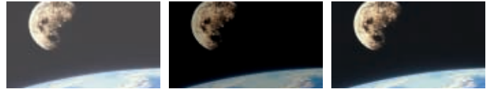
Without lamp power control or dynamic gamma correction blacks and other colours appear lifeless.
