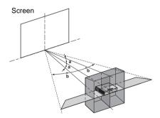
a: Tilting angle of the projector in the "V Keystone" adjustment area
