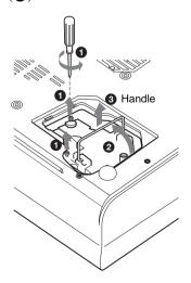
5 Insert the new lamp all the way in until it is securely in place (1). Tighten the two screws (2). Hold down the handle to replace (3).
