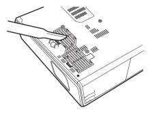
When it becomes difficult to remove the dust from the filter with a vacuum cleaner, remove the air filter and wash it.
