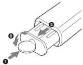
Open the cover (2) with a coin (1) and remove the battery case (3). Install the two size AAA (R03) batteries with the correct polarity.
