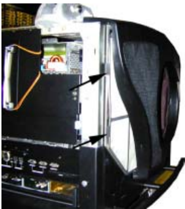
Image C-4 Front side dust filter
