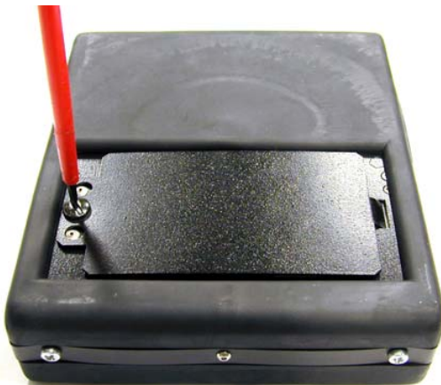
Image 2-13 Open the battery cover
