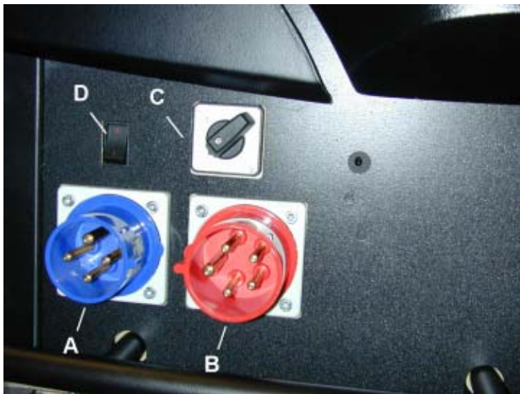
Image 3-1 Possible power connections
