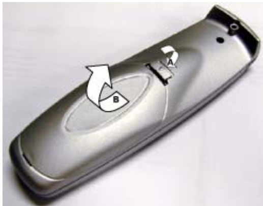
Image 2-10 Battery cover unlock
