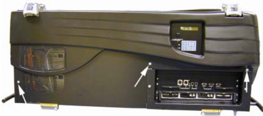
Image 2-7 Removing side cover
