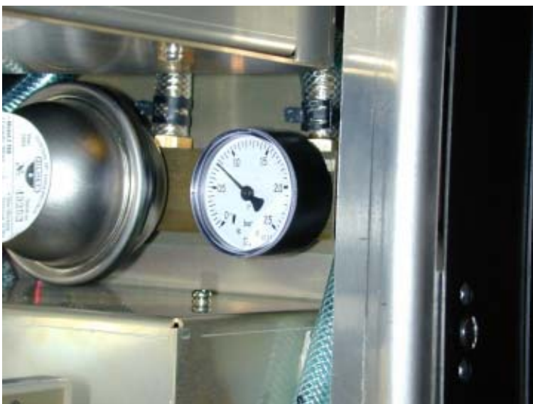
Image 2-9 Cooling liquid pressure
