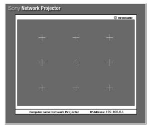
**3** Operate with the mouse of the computer within the projector window displayed on the computer. The operations of the mouse and keyboard reflect those on the projector screen and you can operate the projector.
