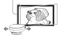
If you position the projector on the left side of the screen, adjust so that the left side of the picture fits the left inside end of the screen frame. With the projector positioned on the right side, adjust so that the right side of the picture fits the right inside end of the screen frame.
