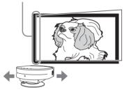
If you position the projector on the left side of the screen, adjust so that the left side of the picture fits the left inside end of the screen frame. With the projector positioned on the right side, adjust so that the right side of the picture fits the right inside end of the screen frame.
