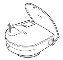
3 Loosen the screw on the lamp unit with a Philips screwdriver. Holding the handle, pull the lamp unit straight up.
