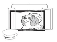
Check that both vertical sides of the picture are parallel to the vertical sides of the screen. If they are not parallel, set "V Keystone" in the INSTALL SETTING menu to "Manual," then press ENTER and adjust the distortion with ↑ or ↓ so that they become parallel.
