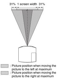
Press the RESET button on the remote control while the Lens Shift adjustment window is displayed, the horizontal position returns to the center of the lens (factory default position). The zoom and focus are not changed.
