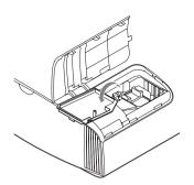
**5** Loosen the 3 screws on the lamp with the Phillips screwdriver. Hold up the handle, then pull the lamp straight out.
