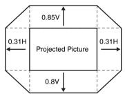
H: Width of the projected picture V: Height of the projected picture
