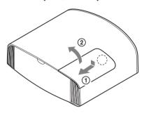
4 Loosen the lamp door (inner cover) screw with a Phillips screwdriver, and then open the lamp door.
