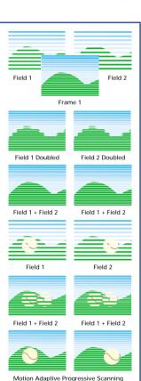
A TV picture comprises of two fields, displayed one after the other, containing the even or odd lines of the image. This only works because CRT phosphors have a persistence that causes them to glow for a short time after the signal is removed.
