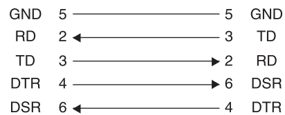
<Projector> (PC serial cable) <Computer>
