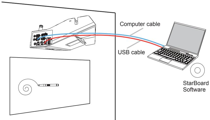
The Interactive Function enables interactive operation without a dedicated board such as the operation on the connected computer or writing on the display with the sensor equipped in the projector and bundled Interactive pen.
