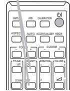
2. The display magnification of the projector switches in order with every press of the **MAGNIFY ON** button.
