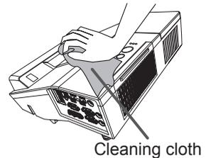
**△ WARNING** ▶ Before caring for the projection window and camera lens, turn the projector off and unplug the power cord, then cool the projector sufficiently.
